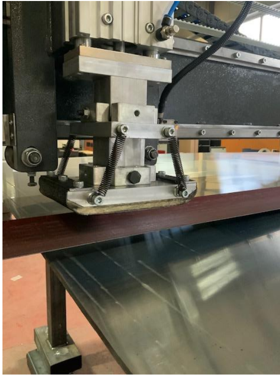
Grinding with Pad Unit
